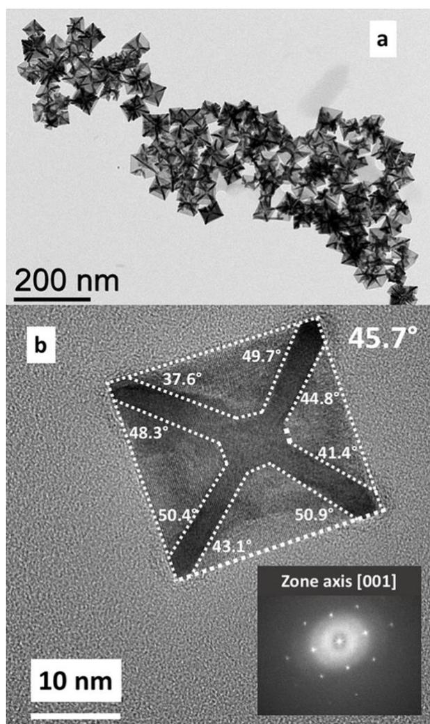
Fig. 1 (a) low magnification TEM micrograph of concave Pt nanocubes obtained at 20°C (1-week reaction). (b) HRTEM of an individual Pt nanocube with the measured dihedral angles, showing a mean angle of 46°; in inset the corresponding Fast Fourier Transform (FFT) of the Pt nanocube oriented along the [001] zone axis.
