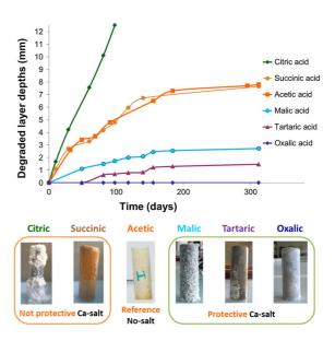
Fig. 1 Kinetics of alteration of various organic acids toward Portland cement paste [26] and aspects of the corresponding specimens. All the acid solutions were 0.28 M and with a pH of 4 (adjusted by addition of soda), except for the oxalic acid solution, the pH of which was 0.85
