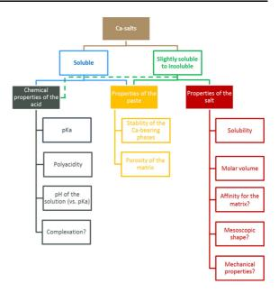
**Fig. 2** Organization chart of parameters influencing the aggressiveness of organic acid toward the cement matrix (from experimental and modeling works). The *dotted line* illustrates secondary influencing parameters (see text)
