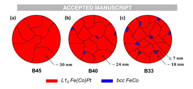
**Figure 10.** Schematic view of the polycrystalline particles for the assemblies (a) B45 (Fe<sub>49</sub>Co<sub>6</sub>Pt<sub>45</sub>), (b) B40 (Fe<sub>48</sub>Co<sub>12</sub>Pt<sub>40</sub>) and (c) B33 (Fe<sub>50</sub>Co<sub>17</sub>Pt<sub>33</sub>) made from *fcc* FePt and *bcc* NPs FeCo after a 1h annealing at 650°C under *forming gas*. (Red :  $LI_0$  Fe(Co)Pt, blue : *bcc* FeCo). The sizes indicate the crystallite mean size deduced from XRD.
