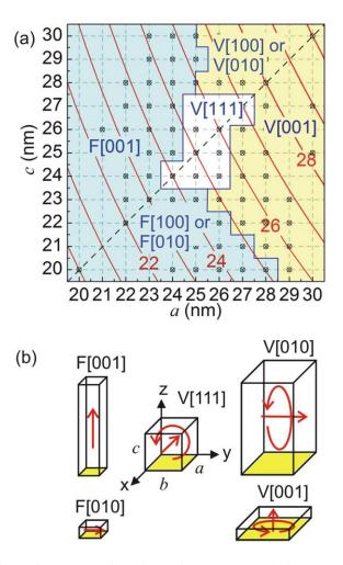
Figure 3. (a) Magnetic configurations as a function of a and c cuboid edge sizes. The background lines correspond to the particle effective size  $t = (a \times a \times c)^{1/3}$  (diagonal dashed line: case of cubes, *i.e.* a=b=c, dots: sizes of simulated cuboids). (b) Sketches of configurations obtained in (a).
