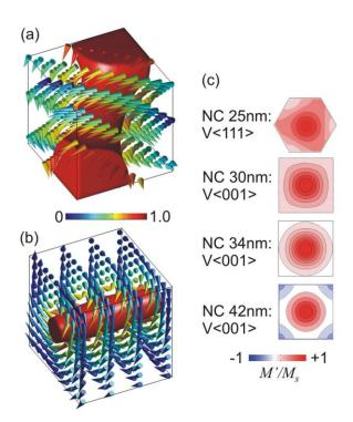
Figure 2. Simulated 3D-magnetic configurations of (a) V<111> (25 nm) and (b) V<001> (30 nm). The red iso-M surface enfolds the magnetic moments whose component along the vortex-axis is  $M'/M_S = 0.8$  ( $M'=M_{III}$  and  $M'=M_{001}$  for V<111> and V<001> resp.). (c) Simulated magnetizations in the median plane (perpendicular to the vortex-axis) for different NC sizes.
