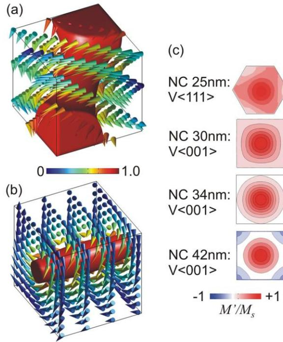
Figure 2. Simulated 3D-magnetic configurations of (a)  $V\langle 111 \rangle$  (25 nm) and (b)  $V\langle 001 \rangle$  (30 nm). The red iso- $M$  surface enfolds the magnetic moments whose component along the vortex-axis is  $M'/M_s = 0.8$  ( $M'=M_{111}$  and  $M'=M_{001}$  for  $V\langle 111 \rangle$  and  $V\langle 001 \rangle$  resp.). (c) Simulated magnetizations in the median plane (perpendicular to the vortex-axis) for different NC sizes.
