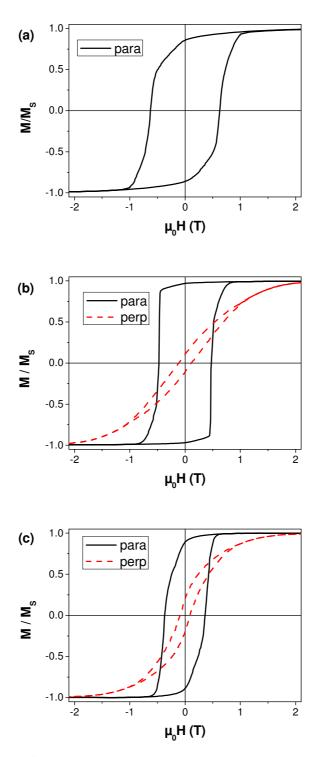
**Figure S2.** M(H) loop of on needle shaped Co NRs assemblies measured with the applied field parallel or perpendicular to the rod alignment direction (a)  $d_m = 10.9$  nm (AR = 18.5); (b)  $d_m = 20.4$  nm (AR = 4.5); (c)  $d_m = 28.3$  nm (AR = 6.7).
