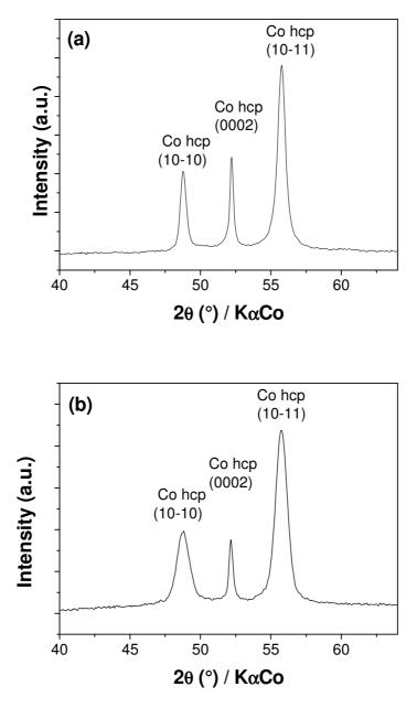
**Figure S1.** Powder X-ray diffraction patterns of cobalt nanorods randomly oriented (a) mean diameter (TEM)  $d_m = 28.3$  nm and mean crystallite size (XRD)  $L_{(10\overline{1}0)} = 26$  nm ; (b) mean diameter (TEM)  $d_m = 10.9$  nm and mean crystallite size (XRD)  $L_{(10\overline{1}0)} = 10$  nm.
