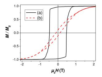
**Figure 3.** Hysteresis loops of an assembly of Co NRs ( $d_m = 20.4$  nm) measured with the applied field parallel (a) or perpendicular (b) to the rod alignment direction.
