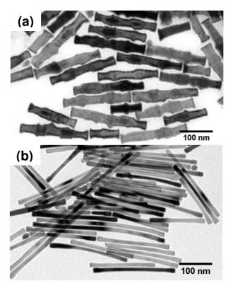
**Figure 1.** TEM micrographs of cobalt nanorods prepared by the up-scale polyol process (5 g of cobalt per batch) under a stirring speed of (a) 160 rpm and (b) 60 rpm. The mean diameter  $(d_m)$  and mean length  $(L_m)$  were determined by measuring 100 rods: (a)  $d_m = 28.3$  nm ( $\sigma = 4.0$  nm),  $L_m = 190$  nm; (b)  $d_m = 10.9$  nm ( $\sigma = 1.1$  nm),  $L_m = 200$  nm.
