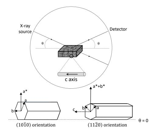
**Figure S4.** Ideal sketch of a nanorod assembly perfectly oriented in the diffraction plane illustrating the absence of (00*l*) reflections in the XRD pattern recorded in  $\theta$ - $\theta$  configuration. At the opposite the intensities of the reflections (1010) and (1120) are expected to be enhanced in comparison with the powder XRD pattern.
