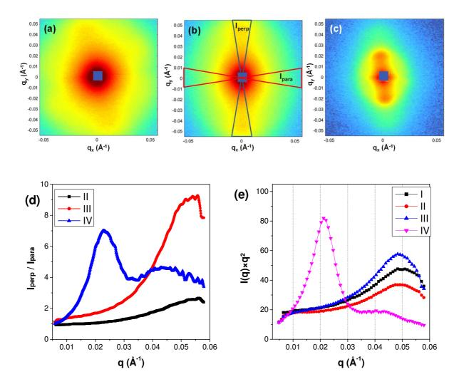
**Figure 5.** SANS pattern of consolidated magnets: (a) magnet II, NRs  $d_m = 10.9$  nm hot compacted at 450 MPa; (b) magnet III, NRs  $d_m = 10.9$  nm cold compacted at 1 GPa; (c) magnet IV, NRs  $d_m = 28.3$  nm hot compacted at 450 MPa ; (d) Anisotropy ratio  $I_{perp}/I_{para}$  for the magnets II, II and IV ; (e) Structure factor  $S(q) = I(q) \times q^2$  for the different magnets, with I(q) the intensity scattered perpendicular to the rods.
