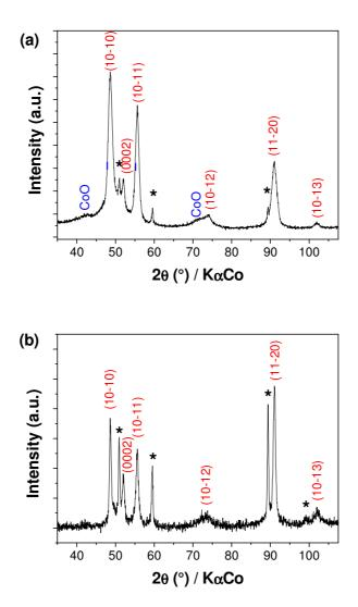
**Figure S3.** X-ray diffraction pattern of consolidated cobalt nanorods measured in  $\theta$ - $\theta$  configuration: (a) Co NRs with a mean diameter of 10.9 nm consolidated under 1 GPa at room temperature (magnet III); (b) Co NRs with a mean diameter of 28.3 nm consolidated under 450 MPa at 180°C (magnet IV). Peaks marked with a (\*) correspond to the sample holder.
