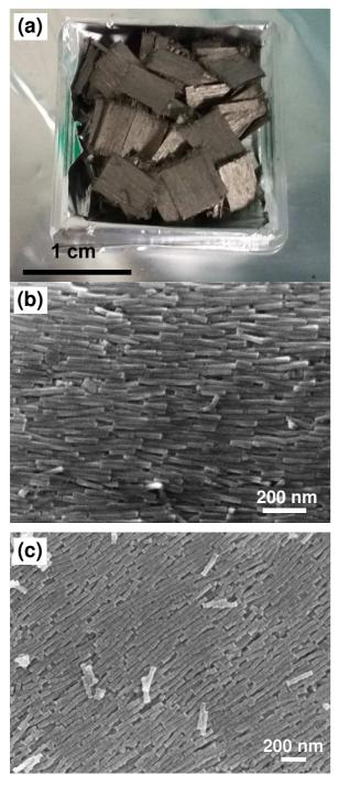
**Figure 2.** (a) Pellets prepared by drying of Co NRs under a magnetic field of 1 T SEM micrographs of the pellets showing the Co NRs alignments: with mean diameter  $d_m = 20.4$  nm (b) and  $d_m = 28.3$  nm (c).
