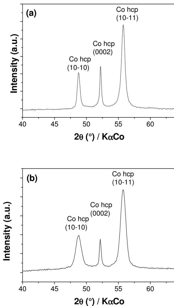
**Figure S1.** Powder X-ray diffraction patterns of cobalt nanorods randomly oriented (a) mean diameter (TEM)  $d_m = 28.3$  nm and mean crystallite size (XRD)  $L_{(10\bar{1}0)} = 26$  nm ; (b) mean diameter (TEM)  $d_m = 10.9$  nm and mean crystallite size (XRD)  $L_{(10\bar{1}0)} = 10$  nm.
