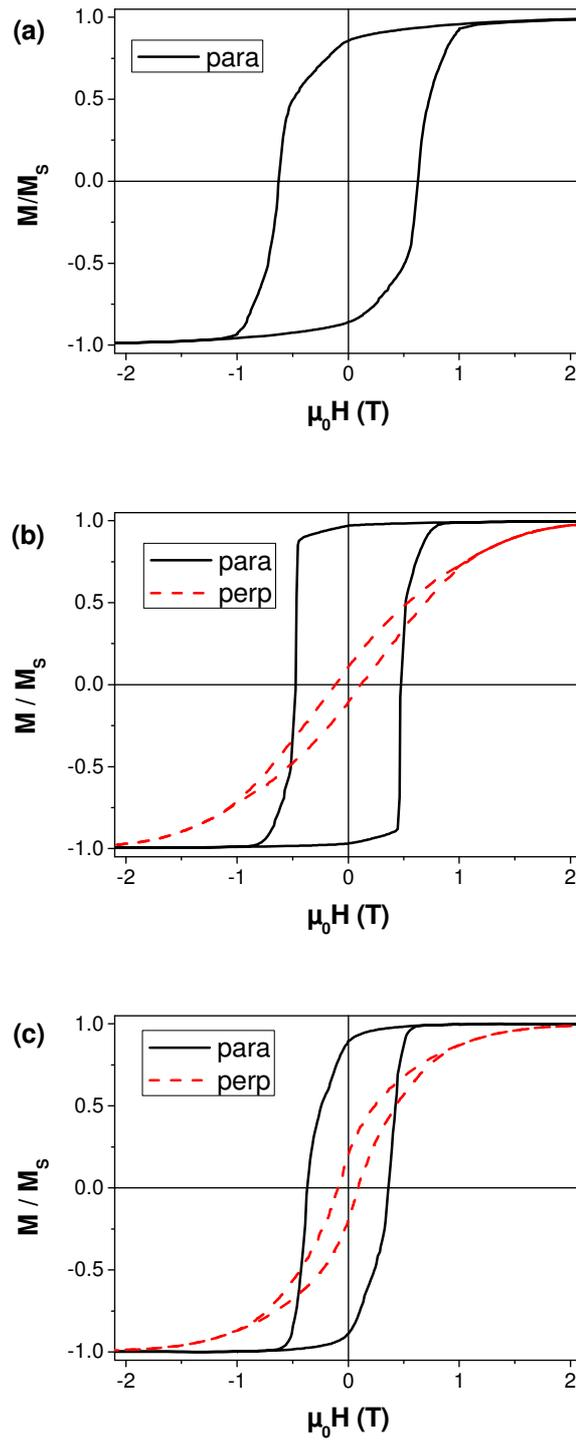
**Figure S2.**  $M(H)$  loop of on needle shaped Co NRs assemblies measured with the applied field parallel or perpendicular to the rod alignment direction (a)  $d_m = 10.9$  nm (AR = 18.5) ; (b)  $d_m = 20.4$  nm (AR = 4.5) ; (c)  $d_m = 28.3$  nm (AR = 6.7).
