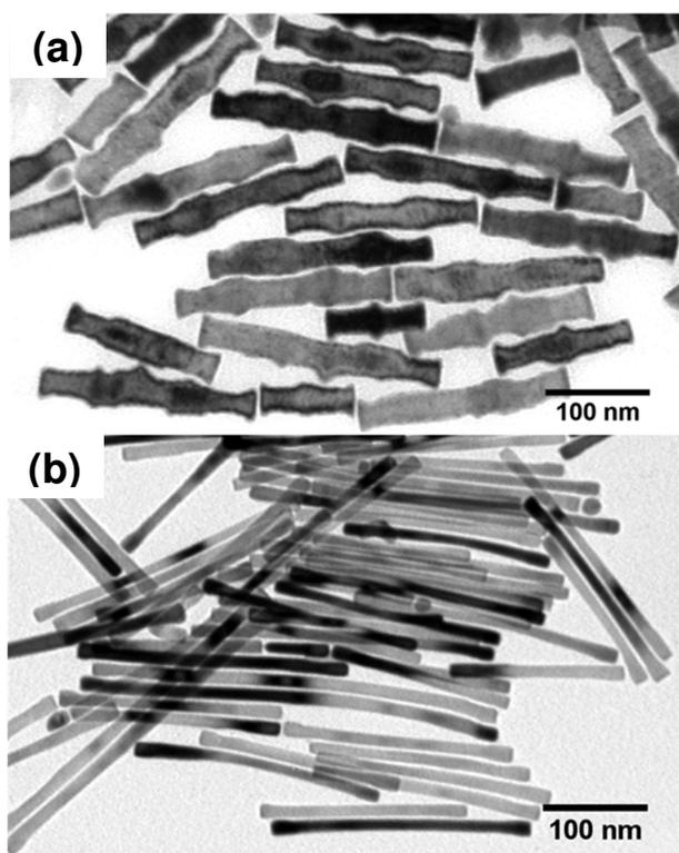
**Figure 1.** TEM micrographs of cobalt nanorods prepared by the up-scale polyol process (5 g of cobalt per batch) under a stirring speed of (a) 160 rpm and (b) 60 rpm. The mean diameter ( $d_m$ ) and mean length ( $L_m$ ) were determined by measuring 100 rods: (a)  $d_m = 28.3$  nm ( $\sigma = 4.0$  nm),  $L_m = 190$  nm; (b)  $d_m = 10.9$  nm ( $\sigma = 1.1$  nm),  $L_m = 200$  nm.
