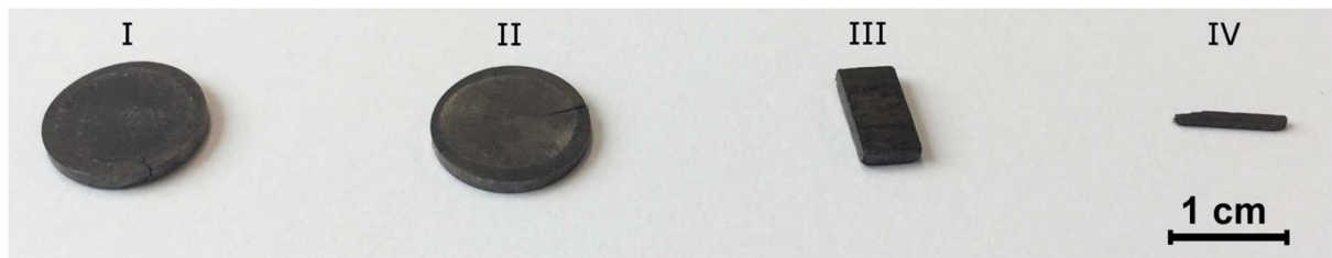
Figure 4. Images of consolidated Co nanowires in different shapes. d_m = 10.9 nm compacted at 300 MPa, 180°C (I) ; 450 MPa, 180°C (II); 1GPa, RT (III) ; and d_m = 28.3 nm compacted at 450 MPa, 180°C (IV).
