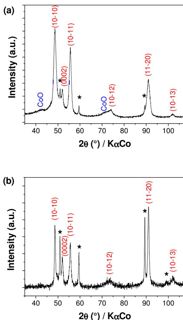
**Figure S3.** X-ray diffraction pattern of consolidated cobalt nanorods measured in  $\theta$ - $\theta$  configuration: (a) Co NRs with a mean diameter of 10.9 nm consolidated under 1 GPa at room temperature (magnet III); (b) Co NRs with a mean diameter of 28.3 nm consolidated under 450 MPa at 180 $^\circ\text{C}$  (magnet IV). Peaks marked with a (\*) correspond to the sample holder.
