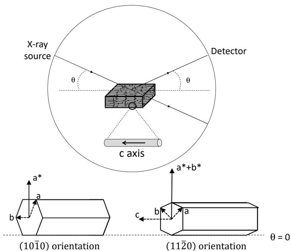
**Figure S4.** Ideal sketch of a nanorod assembly perfectly oriented in the diffraction plane illustrating the absence of  $(00l)$  reflections in the XRD pattern recorded in  $\theta$ - $\theta$  configuration. At the opposite the intensities of the reflections  $(10\bar{1}0)$  and  $(11\bar{2}0)$  are expected to be enhanced in comparison with the powder XRD pattern.
