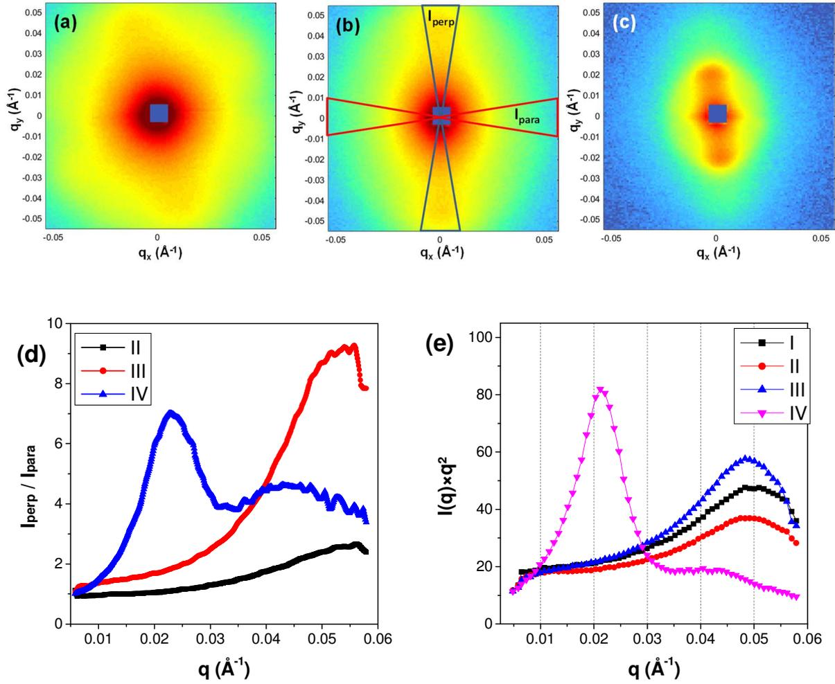
**Figure 5.** SANS pattern of consolidated magnets: (a) magnet II, NRs  $d_m = 10.9$  nm hot compacted at 450 MPa; (b) magnet III, NRs  $d_m = 10.9$  nm cold compacted at 1 GPa; (c) magnet IV, NRs  $d_m = 28.3$  nm hot compacted at 450 MPa ; (d) Anisotropy ratio  $I_{\text{perp}}/I_{\text{para}}$  for the magnets II, II and IV ; (e) Structure factor  $S(q) = I(q) \times q^2$  for the different magnets, with  $I(q)$  the intensity scattered perpendicular to the rods.
