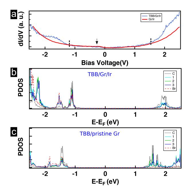
Figure 5: (a) Spatially averaged tunneling spectra recorded over Gr/Ir and on a monolayer of 4MOL polymorph on Gr/Ir(111). The arrow points at the Gr/Ir surface state. Projected densities of states (PDOS) of one single TBB molecule adsorbed (b) on a FCC site of Gr/Ir(111) and (c) on pristine Gr. PDOS are projected on different rings 1, 2, 3 and C as labelled in Fig. 1(d) and on bromine atoms.
