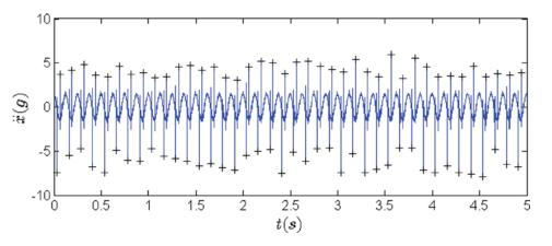
Fig. 4 Acceleration of LO with b = 9 mm: impact moments are denoted by crosses
