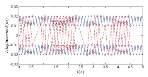
Fig. 9 Reconstruction of the displacement of VI NES in dotted curve with b = 15 mm: displacement of LO in sine curve is shifted to negative and positive by b and impact moments are denoted by circles
