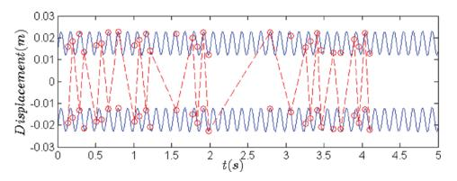
Fig. 11 Reconstruction of the displacement of VI NES in dotted curve with b = 17.5 mm: displacement of LO in sine curve is shifted to negative and positive by *b* and impact moments are denoted by circles
