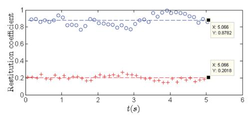
Fig. 16 Estimated restitution coefficients at the right side in circles and the left side in crosses with b = 9 mm: dotted lines are two corresponding values of root-mean-square
