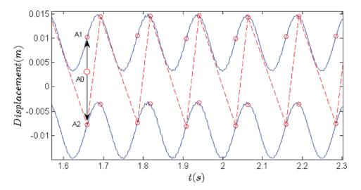
Fig. 7 Reconstruction of the displacement of VI NES in dotted curve with b = 9 mm: displacement of LO in sine curve is shifted to negative and positive by *b*, and impact moments are denoted by circles
