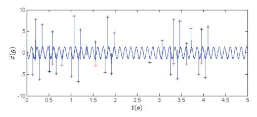
Fig. 10 Acceleration of LO with b = 17.5 mm: impact moments are denoted by crosses
