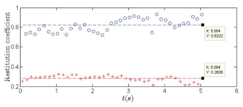
Fig. 17 Estimated restitution coefficients at the right side in circles and the left side in crosses with b = 7.5 mm: dotted lines are two corresponding values of root-mean-square
