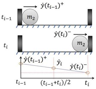
Fig. 15 Schema of corrected velocities after and before impacts
