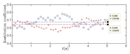
Fig. 18 Estimated restitution coefficients at the right side in circles and the left side in crosses with b = 6 mm: dotted lines are two corresponding values of root-mean-square
