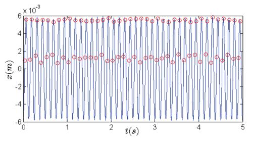
Fig. 6 Displacement of LO with b = 9 mm: impact moments are denoted by circles
