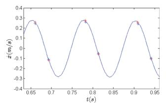
Fig. 14 Velocity of LO before and after impact in crosses with b = 9 mm
