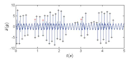
Fig. 8 Acceleration of LO with b = 15 mm: impact moments are denoted by crosses [10]
