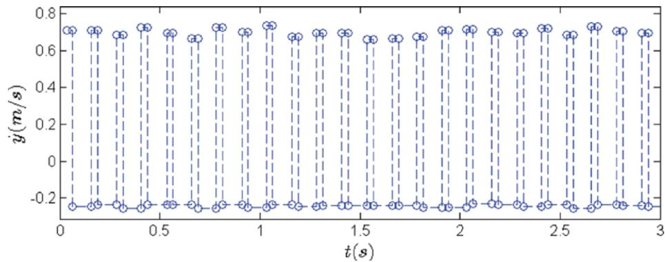
Fig. 12 Velocity of VI NES with  $b = 9$  mm: impact moments are denoted by circles
