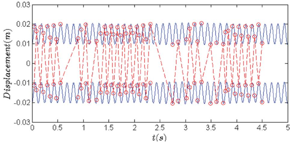
Fig. 9 Reconstruction of the displacement of VI NES in dotted curve with  $b = 15$  mm: displacement of LO in sine curve is shifted to negative and positive by  $b$  and impact moments are denoted by circles
