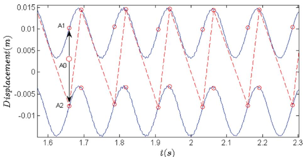
**Fig. 7** Reconstruction of the displacement of V NES in dotted curve with  $b = 9$  mm: displacement of LO in sine curve is shifted to negative and positive by  $b$ , and impact moments are denoted by circles
