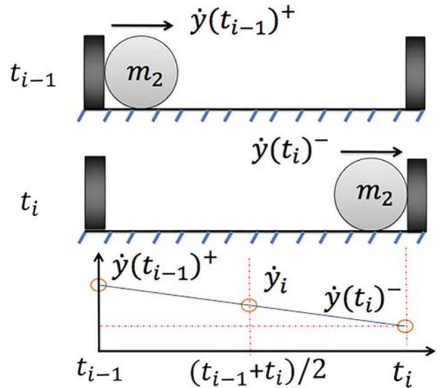
Fig. 15 Schema of corrected velocities after and before impacts
