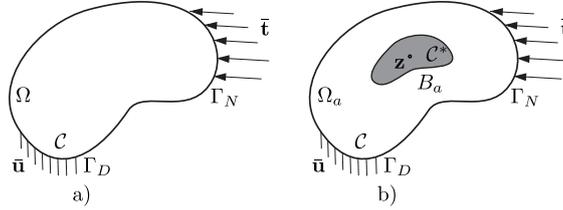
Figure 1: Model scheme showing the geometric setting, that is, unperturbed a) and perturbed b) domains,  $\Omega$  and  $\Omega_a$ , respectively. The inhomogeneity  $B_a$  located at  $\mathbf{z}$  is the shaded subdomain in (b).
