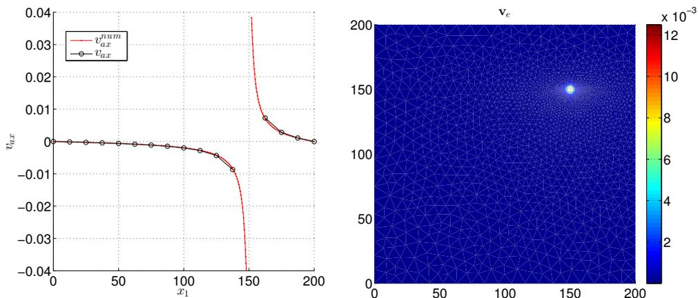
Figure 5: The comparison of the asymptotic approximation  $\mathbf{v}_a$  and reference solution  $\mathbf{v}_a^{num}$ , along crosssection  $A - A$  (left), and in terms of contour plot of perturbation error  $\mathbf{v}_e$  (right). Both are given for a membrane with a circular hole on site  $\mathbf{z}$  of radius  $a = 2$  mm.
