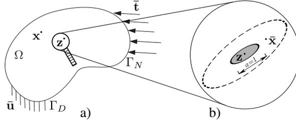
Figure 2: Scheme showing the *far-field* a) and *near-field* b) expansions. Far-field is represented with coordinates at the structure scale, while the near-field represents zoom on the inhomogeneity represented by coordinates at the structure scale.
