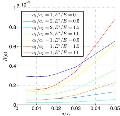
Figure 6: The plot of discrepancy versus the normalized inhomogeneity size. The soft and hard inclusions with elliptic and circular shape are considered.
