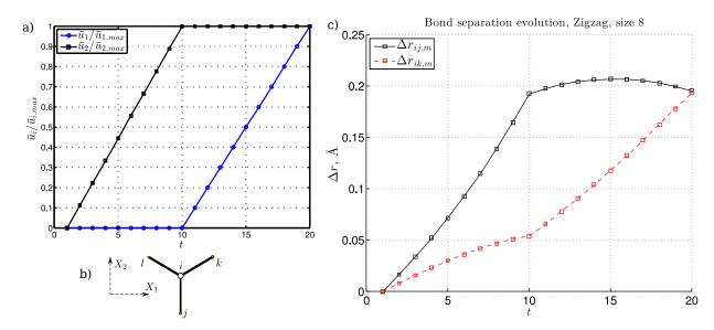
**Figure 6:** Load program showing the given displacements (upper and right edges) with respect to the pseudo time a), and b) the bulk atom *i* with its neighbourhood. The given load program causes the lattice deformation as presented in c). Due to symmetry, the bond separation  $\Delta r_{il}$  is equal as  $\Delta r_{ij}$ , and is thus omitted.
