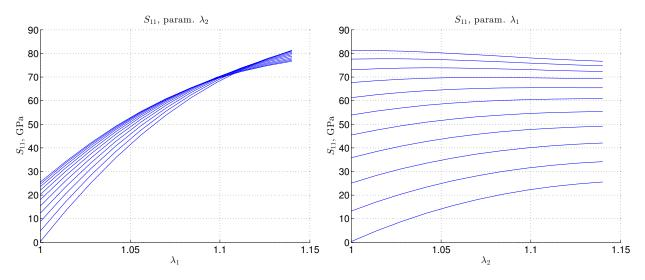
Figure 5: The stress-stretch plots showing the component  $S_{11}$  versus: stretch  $\lambda_1$  with parameter  $\lambda_2$  (left plot), and stretch  $\lambda_2$  with parameter  $\lambda_1$  (right plot). The parameter is in the range  $\lambda_i = 1, ..., \overline{\lambda}$ , where the lower-most stress curve corresponds to the value of the paremeter  $\lambda_i = 1$ , while the upper-most corresponds to  $\lambda_i = \overline{\lambda}$ .
