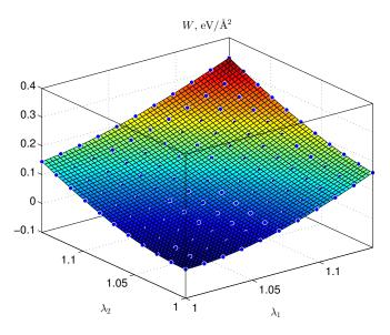
Figure 2: The surface plot of the strain energy density polynomial surface fit  $W_{\text{fit}}(\lambda_1, \lambda_2)$ . The fit is obtained by means of series of biaxial tests performed by molecular mechanics simulation  $(\hat{W}(\lambda_1, \lambda_2))$  represented with circular markers on the grid  $0 \le \bar{\lambda}_i \le 1.15$ , i = 1, 2.
