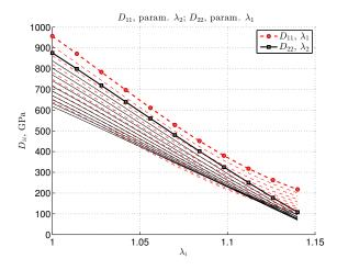
Figure 7: Evolution of the diagonal components of the reduced tangent elastic modulus with the associated stretches. The thick lines with markers denote the evolution of  $D_{ii}$  without pre-stretch.
