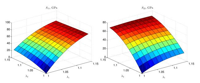
Figure 3: Surface plot of the nonzero stress components vs. principal stretches.
