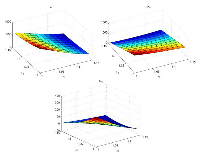
Figure 4: Surface plot of the components of reduced tangent elastic modulus. The values are given in GPa.
