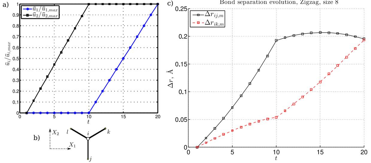
**Figure 6:** Load program showing the given displacements (upper and right edges) with respect to the pseudo time a), and b) the bulk atom  $i$  with its neighbourhood. The given load program causes the lattice deformation as presented in c). Due to symmetry, the bond separation  $\Delta r_{il}$  is equal as  $\Delta r_{ij}$ , and is thus omitted.
