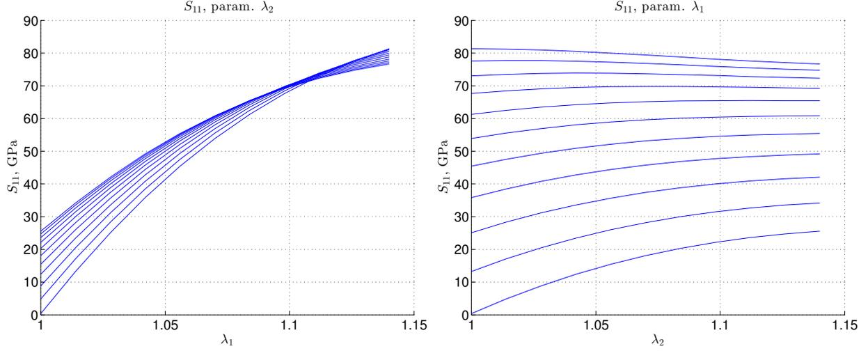
**Figure 5:** The stress-stretch plots showing the component  $S_{11}$  versus: stretch  $\lambda_1$  with parameter  $\lambda_2$  (left plot), and stretch  $\lambda_2$  with parameter  $\lambda_1$  (right plot). The parameter is in the range  $\lambda_i = 1, \dots, \bar{\lambda}$ , where the lower-most stress curve corresponds to the value of the parameter  $\lambda_i = 1$ , while the upper-most corresponds to  $\lambda_i = \bar{\lambda}$ .
