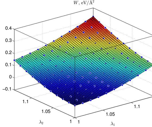
**Figure 2:** The surface plot of the strain energy density polynomial surface fit  $W_{\text{fit}}(\lambda_1, \lambda_2)$ . The fit is obtained by means of series of biaxial tests performed by molecular mechanics simulation ( $\dot{W}(\lambda_1, \lambda_2)$ ) represented with circular markers on the grid  $0 \leq \bar{\lambda}_i \leq 1.15$ ,  $i = 1, 2$ .
