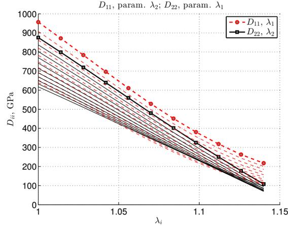
**Figure 7:** Evolution of the diagonal components of the reduced tangent elastic modulus with the associated stretches. The thick lines with markers denote the evolution of  $D_{ii}$  without pre-stretch.
