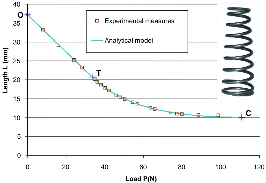
**Fig. 7** Experimental data and analytical model of two constant pitch conical springs, #1 is telescoping, #2 is non-telescoping
