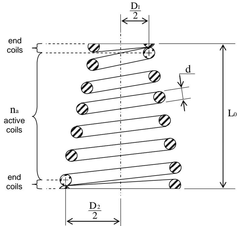
**Fig. 1 Parameters of the studied conical spring**
