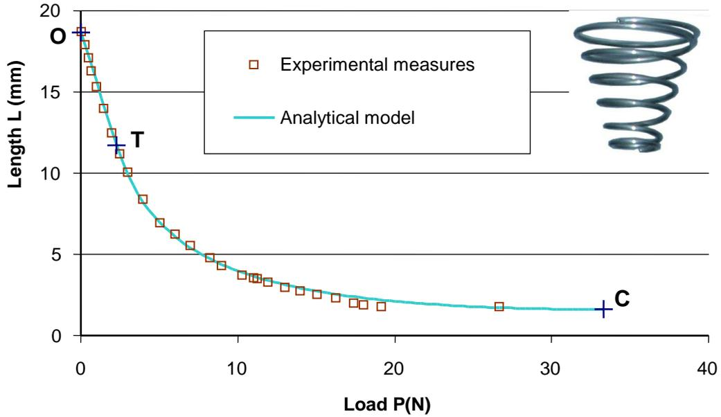
**#2 - Non-telescoping conical spring**
