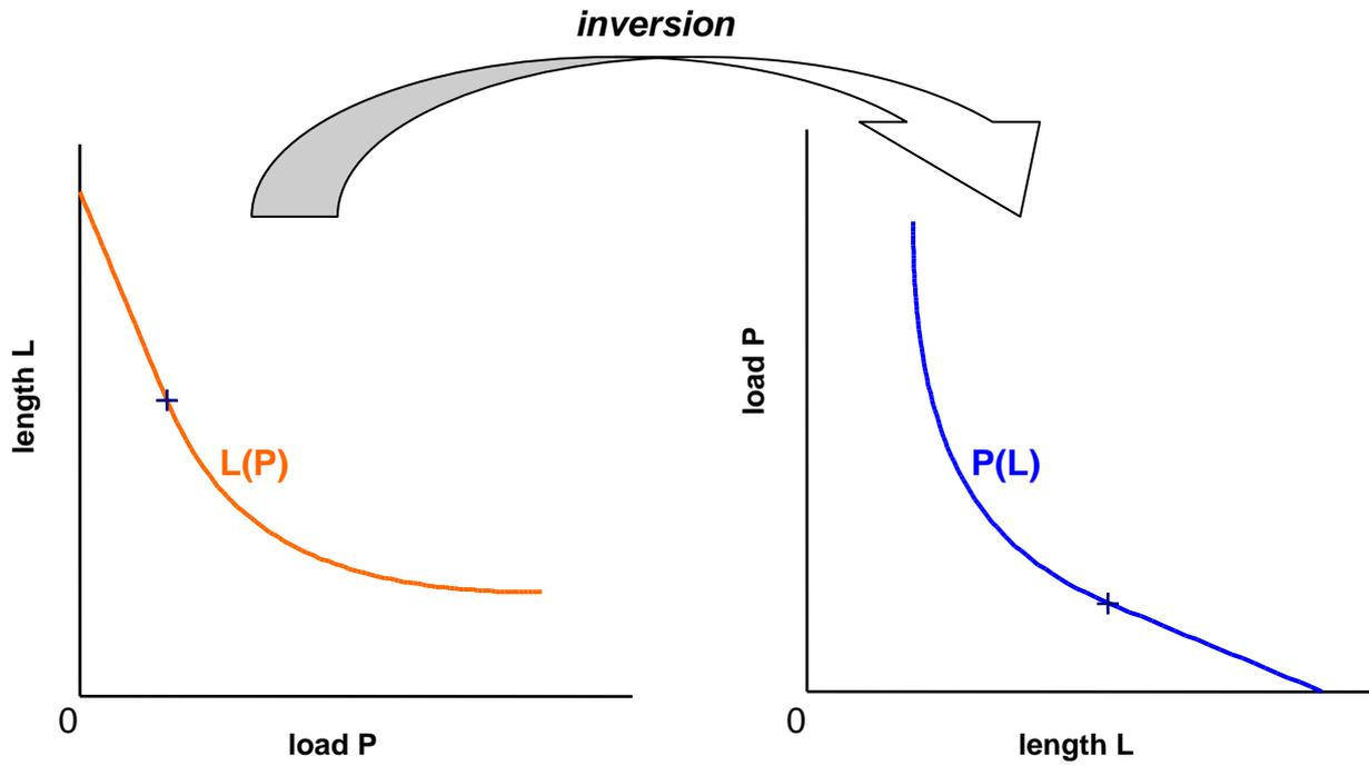
Fig. 5 Graphic representations of  $L(P)$  and its inverse  $P(L)$  for the same conical spring
