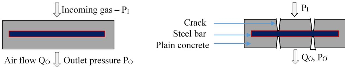
**Fig. 2:** Reinforced concrete for  $Q_O$  measurement: case n°1
