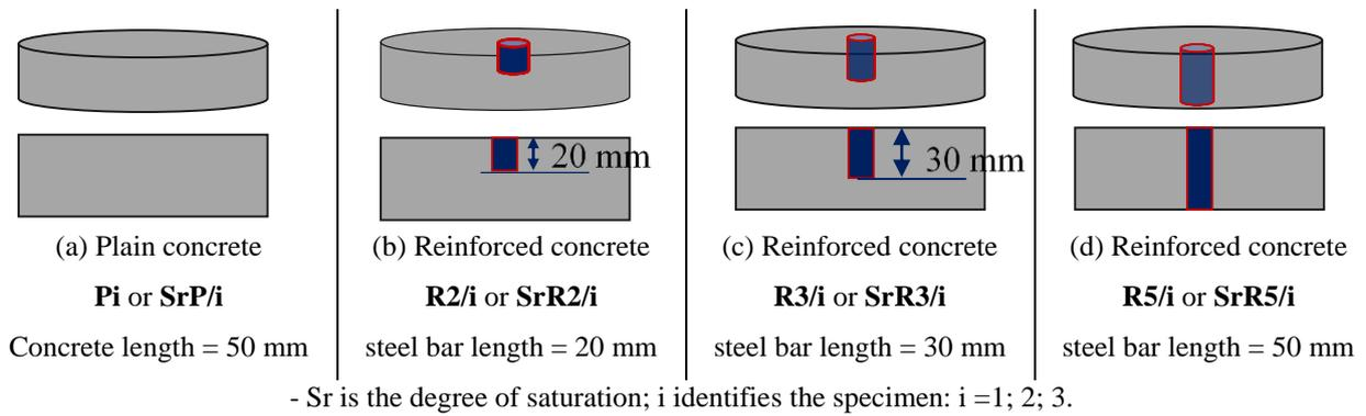
**Fig. 4:** Types and codes of specimens
