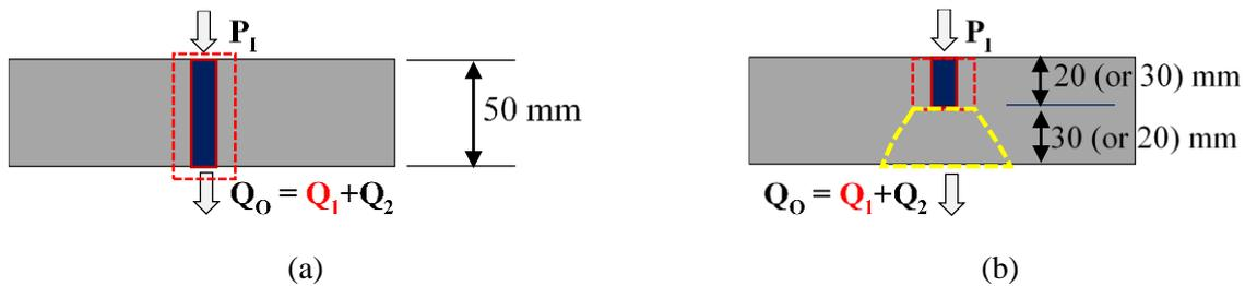
Legend.  $Q_0$  = Total air flow;  $Q_2$  = flow through concrete only;  $Q_1$  = flow through the defect
