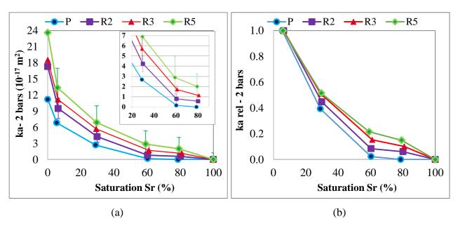
**Fig. 7**: Apparent permeability (a) and relative permeability  $k_{Sr}/k_{Sr=6\%}$  (b) for  $P_I = 2$  bars
