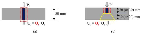
Legend.  $Q_0$  = Total air flow;  $Q_2$  = flow through concrete only;  $Q_1$  = flow through the defect **Fig. 11:** Permeability zones in R5 (a) and permeability zones in R2 and R3 (b)
