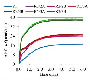
Fig. 6: Air flow Q(t) – two faces (A and B), tested at the saturation degree equal to 0% for the
