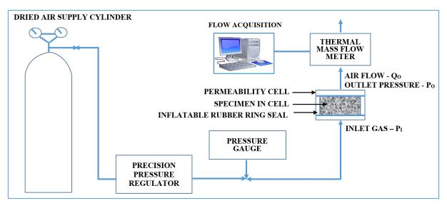
Fig. 1: Experimental apparatus
