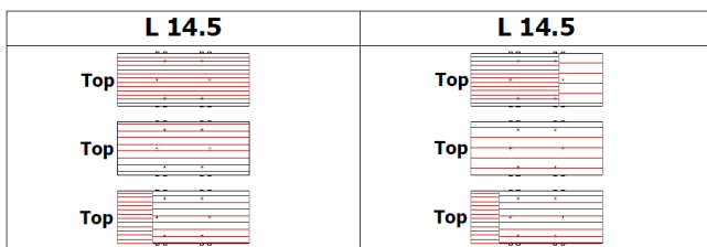
Figure 13. Orientation of cracks and density (a.), of plain stress-free (b.), of reinforced specimens (c.), of specimens reinforced and with stirrups (d.), and prestressed specimens (e.) after 336 days of immersion.
