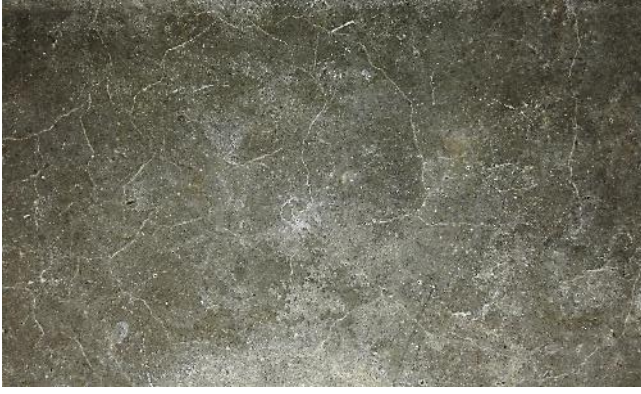
Figure 12. Example of cracking patterns of the specimens.
