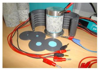
Fig. 3 Resistivity cell
