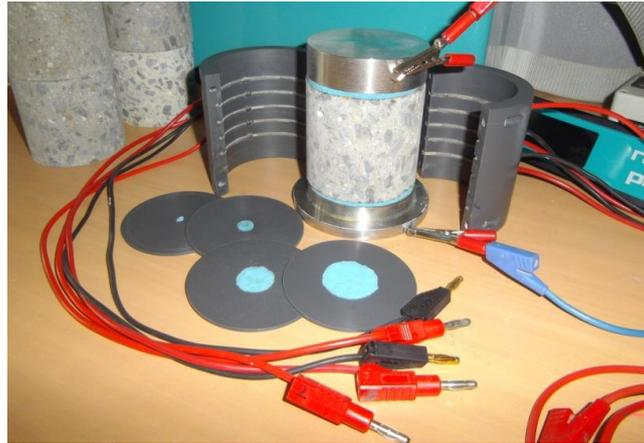
Fig. 3 Resistivity cell
