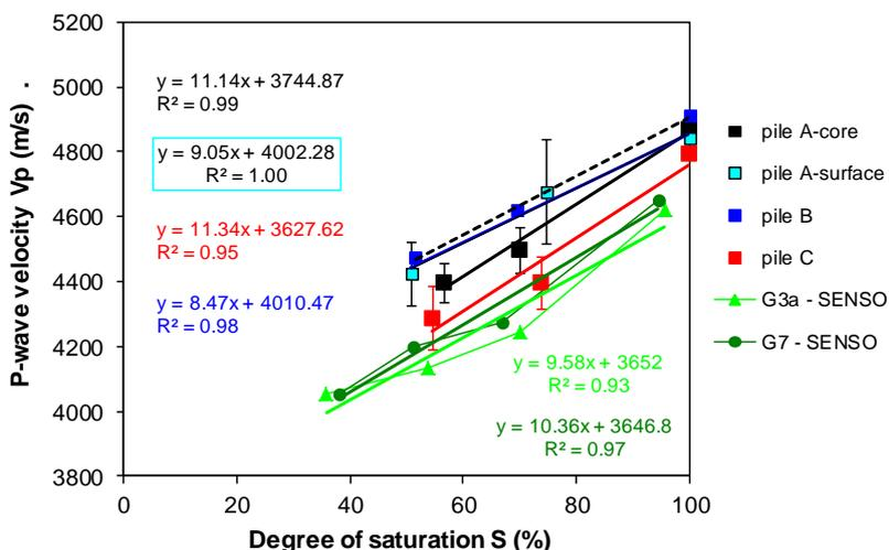
Fig. 7 P-wave velocity vs. degree of saturation for Marly cores and ANR-SENSO slabs
