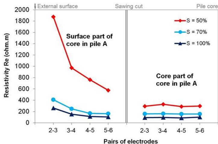
Fig. 10 Resistivity of pairs of annular electrodes for two parts of a core taken in Pile A either the part near the surface ( $0 \text{ mm} \leq \text{depth} \leq 70 \text{ mm}$ ) or the part in the pile core (approx.  $75 \text{ mm} \leq \text{depth} \leq 145 \text{ mm}$ )
