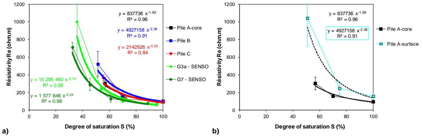
Fig. 9 Resistivity vs. degree of saturation for Marly cores and ANR-SENSO slabs - a) cores from the pile core - b) Pile A: cores from the core and the surface
