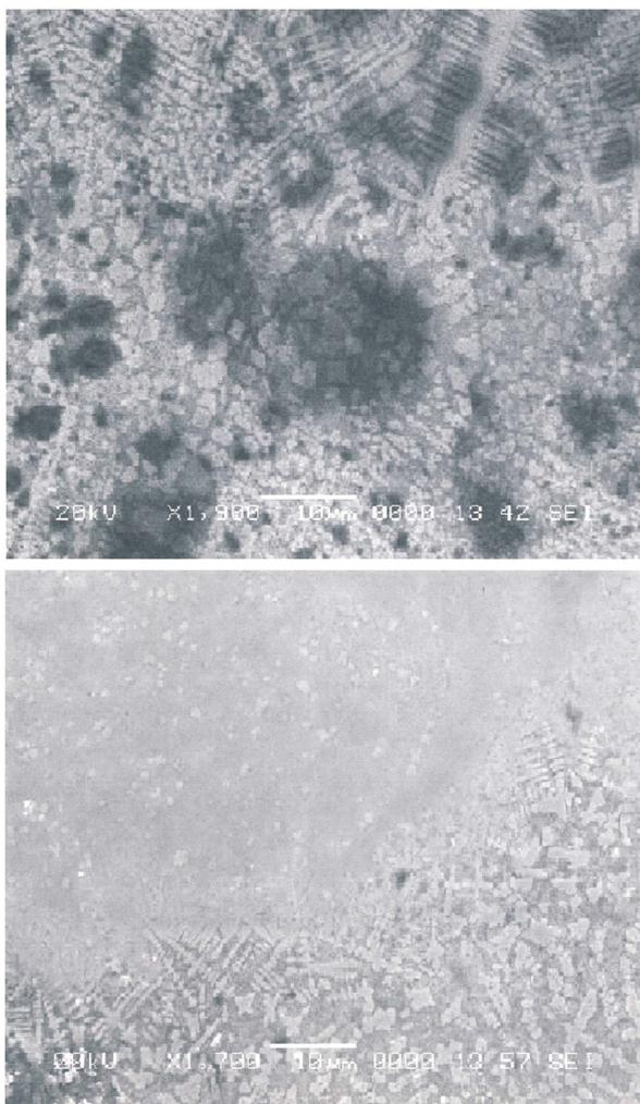
**Figure 2** | Dendritic solidification of Inconel 625 in the region close to the melt pool<sup>16</sup>.
