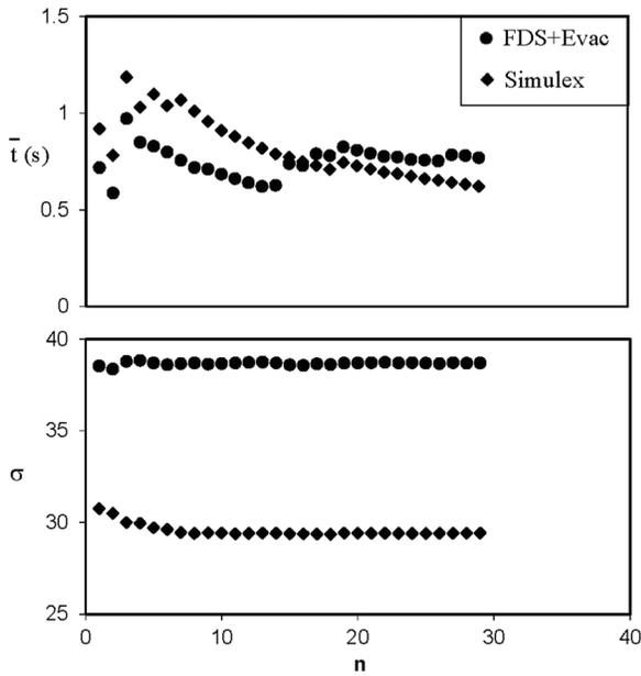
FIG. 4. The effect of the number of simulations of one evacuation scenario on the average evacuation time  $\bar{t}$  and the standard deviation (from the case with hall aspect ratio being 1.21) in the configuration of Fig. 3(b).
