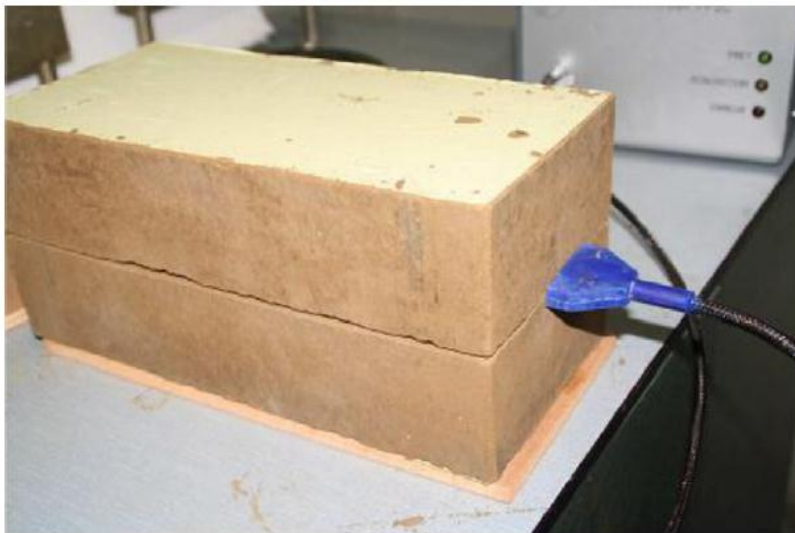
Fig. 4. Procedure to measure the thermal conductivity on PABs.
