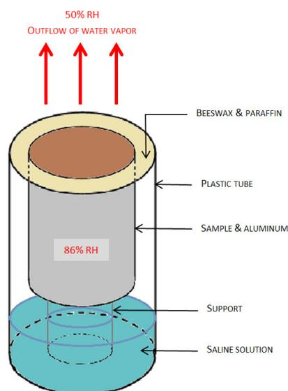
**Fig. 2.** Schematic diagram of the wet cup.
