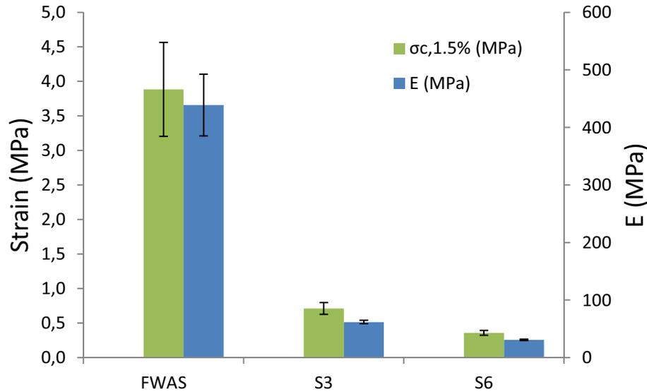
**Fig. 4.** Compressive strength at 1.5% strain ( $\sigma_{c,1.5\%}$ ) and Young's modulus with friction at the plate- specimen interface
