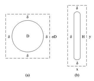
FIG. 7. Uniform spacings around tubes (round, flat) in an array.
