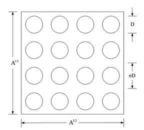
FIG. 4. Square array of horizontal cylinders.
