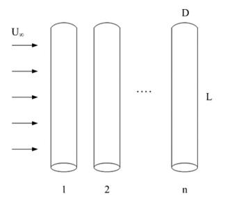
FIG. 8. Row of parallel tubes in cross flow.
