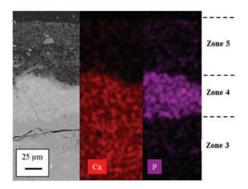
**Fig. 8.** SEM observation in BSE mode and chemical mapping of calcium (Ca) and phosphorus (P) EDS in the outer zones (zones 3 to 5 as defined in Fig. 6) of an ordinary cement paste immersed in solid/liquid phase of biowaste in anaerobic digestion conditions for 4 weeks.
