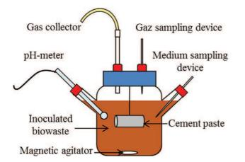
Fig. 3. Schematic representation of the anaerobic bioreactors placed on a magnetic plate for mixing purposes and kept in an oven regulated at 37  $^\circ$ C.
