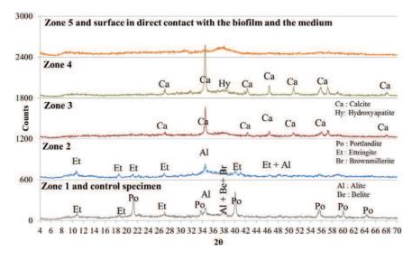
Fig. 9. Mineralogical analyses by XRD of ordinary cement paste immersed in the solid/liquid phase of biowaste in anaerobic digestion conditions for 4 weeks.
