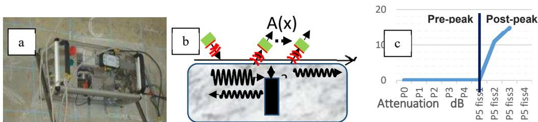
**FIGURE 4.** a) Ultrasonic surface waves scanner [20] b) Principle, c) Attenuation of the surface waves
