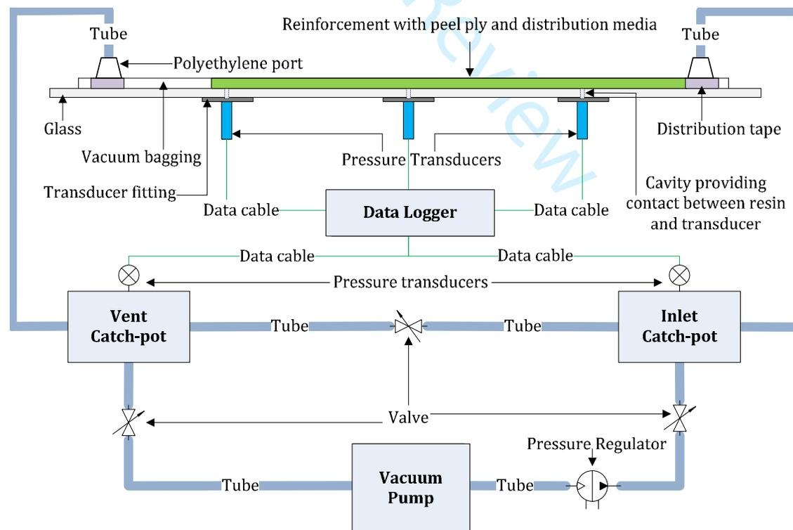
Figure 5: Schematic of the Resin Infusion setup
