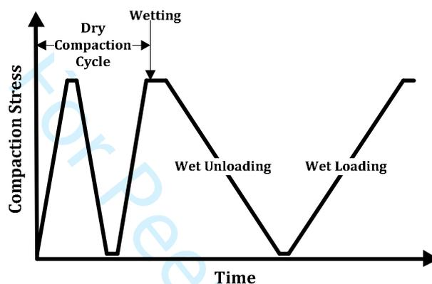
Figure 3: Schematic of compaction cycle for material characterization
