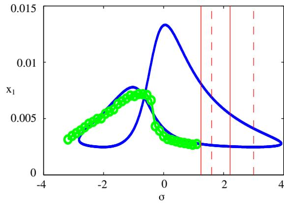
Fig. 10. Experimental and analytical frequency response curves of the LO for  $G = 0.16mm$  ( $A = 0.019$ ). Blue lines corresponds to the analytical prediction, green lines represents the experimental measurements. Straight and dashed red lines denotes the experimentally and numerically found SMR zone.
