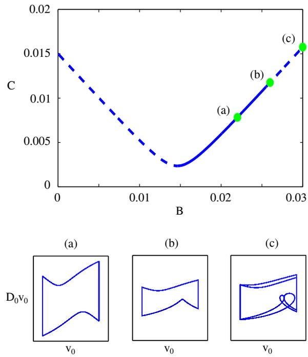
Fig. 3. SIM of the problem for  $r = 0.6$ ,  $\Delta = 0.015$ . Straight and dotted lines denotes stable and unstable branch of the SIM respectively. Numerical phase space : (a) stable symmetric 1 : 1 motion, (b) asymmetric 1 : 1 motion, (c) asymmetric 2 : 2 motion.
