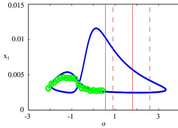
Fig. 12. Experimental and analytical frequency response curve of the LO for  $G = 0.14mm$  ( $A = 0.017$ ). Blue lines corresponds to the analytical prediction, green lines represents the experimental measurements. Straight and dashed red lines denotes the experimentally and numerically found SMR zone.
