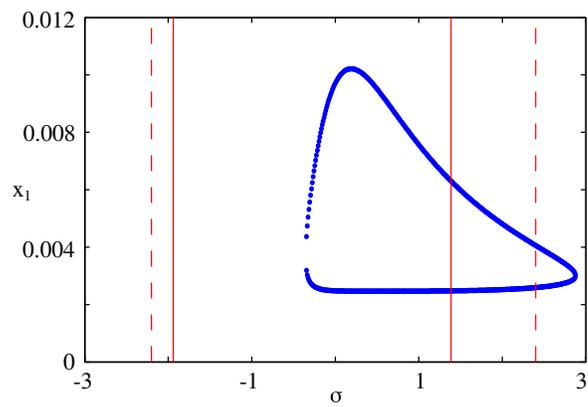
Fig. 13. Analytical frequency response curve of the LO for  $G = 0.125mm$  ( $A = 0.015$ ). Blue lines corresponds to the analytical prediction. Straight and dashed red lines denotes the experimentally and numerically found SMR zone.
