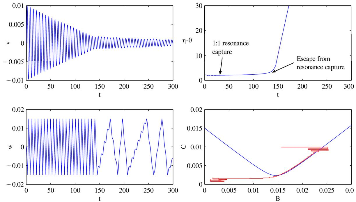
Fig. 4. Illustration of the process of TET under transient loading for  $\lambda = 0.95$ ,  $\varepsilon = 0.84\%$ ,  $\Delta = 0.015$ . (a, b) : result of numerical integration , (c) : 1 : 1 resonance capture and (d) : projection of the result of numerical integration on the SIM.
