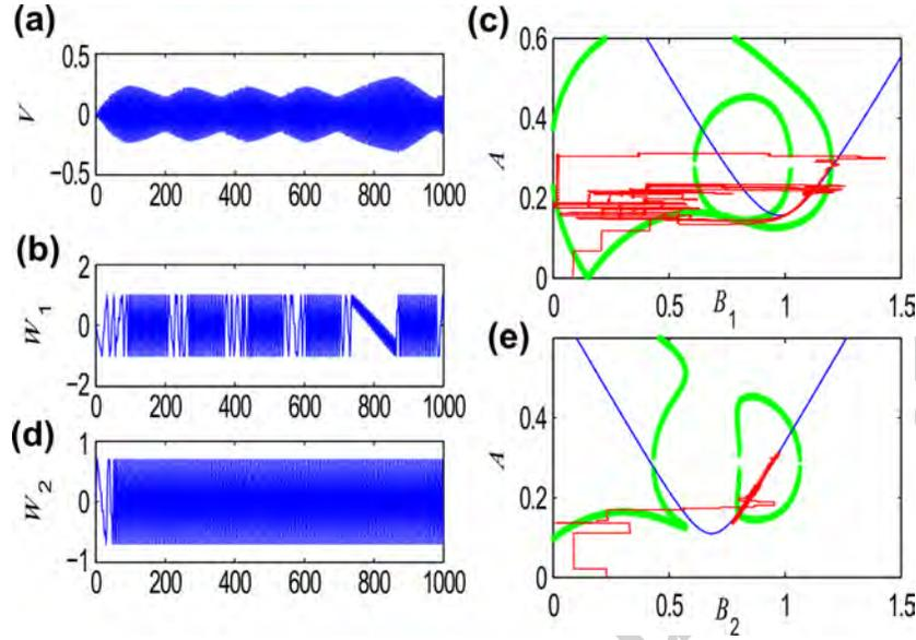
**Fig. 2.** Numerical integration of Eqs. (7, 8) for  $G = 0.8$  and  $\sigma = 0.5$ : (a) SMR of  $V$ ; (b) intermittent resonance of  $W_1$  related to the first VI NES; (c) the analytically obtained SIM of the first order in blue curve and of the second order in green curve, the projection of motion for the first VI NES in red curve; (d) the constant response of  $W_2$  related to the second VI NES; (e) the projection of motion for the second VI NES in red curve.
