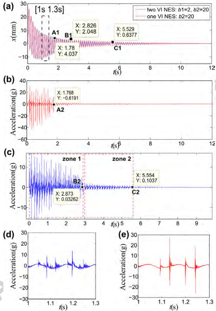
**Fig. 10.** Response comparison between LO coupled with one VI NES and two VI NES: (a) an imposed time history of displacement; (b) a time history of acceleration with one VI NES; (c) a time history of acceleration with two VI NES; (d) a detailed view of one period of acceleration with two VI NES; (e) a detailed view of one period of acceleration with one VI NES.
