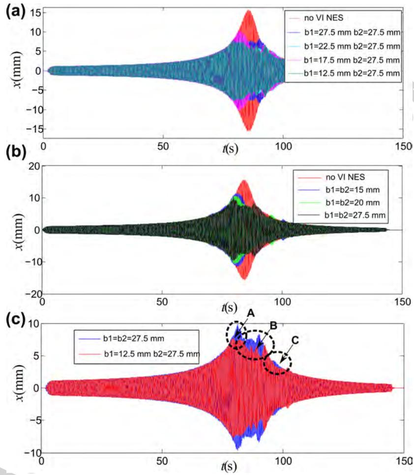
**Fig. 8.** Responses of LO during the sweep experiments and efficiency comparison: (a) with different  $b_1$  and  $b_2$ ; (b) with the same  $b_1$  and  $b_2$ ; (c) the efficiency comparison for two relative optimal cases.
