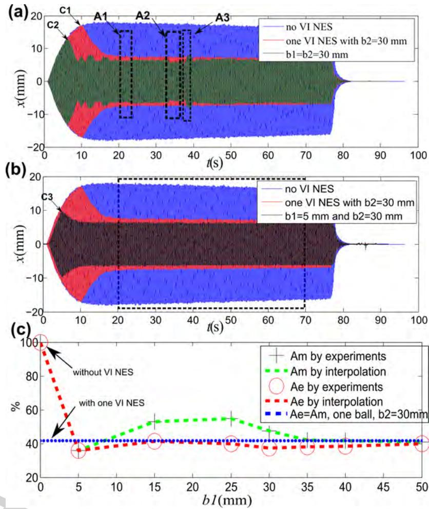
**Fig. 6.** Typical response regimes and their efficiency comparison with different combinations of clearances: (a-b) response regimes; (c) efficiency comparison by average and maximal amplitude ratios ( $A_e$  and  $A_m$ ).
