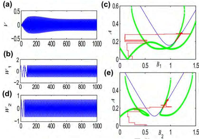
**Fig. 3.** Numerical integration of Eqs. (7, 8) for  $G = 0.9$  and  $\sigma = -0.2$ : (a) steady state response of  $V$ ; (b) constant resonance of  $W_1$  related to the first VI NES; (c) the analytically obtained SIM of the first order in blue curve and of the second order in green curve, the projection of motion for the first VI NES in red curve; (d) the constant response of  $W_2$  related to the second VI NES; (e) the projection of motion for the second VI NES in red curve.
