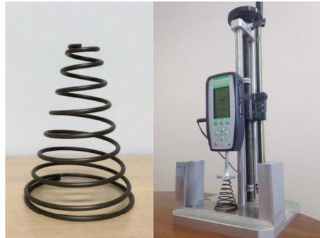
Fig. 12. Conical spring manufactured and measuring equipment
