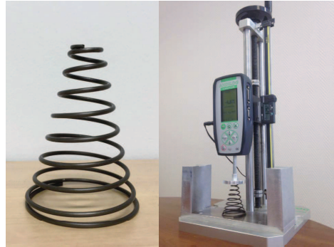
Fig. 12. Conical spring manufactured and measuring equipment
