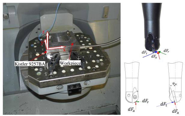
Fig. 7 Cutting force experimental setup
