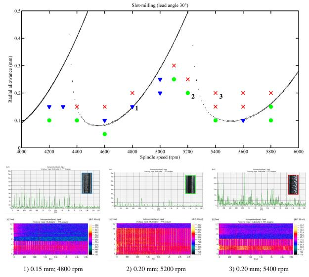
Fig. 11 Experimental stability for slot-milling (lead angle 30°), stable tests results are marked with green  $\circ$ , limited stable tests results are marked with blue  $\nabla$ , unstable tests results are marked with red  $\times$
