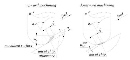
Fig.3 Difference between radial allowance and axial depth of cut in a case of inclined surface ball end milling
