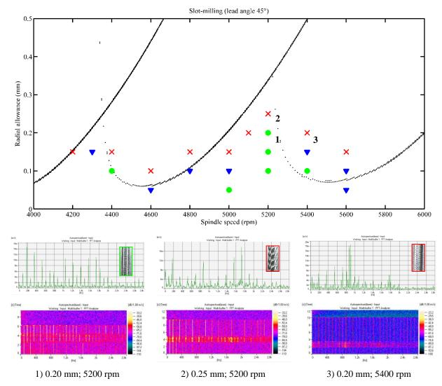
Fig. 12 Experimental stability for slot-milling (lead angle 45°), stable tests results are marked with green  $\circ$ , limited stable tests results are marked with blue  $\nabla$ , unstable tests results are marked with red  $\times$
