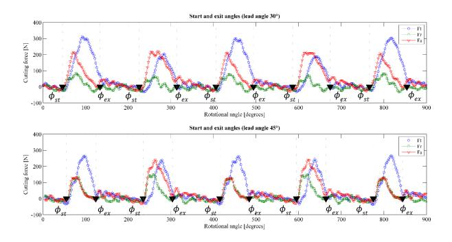
Fig. 8 Tangential (blue line), radial (green line) and axial (red line) cutting force components
