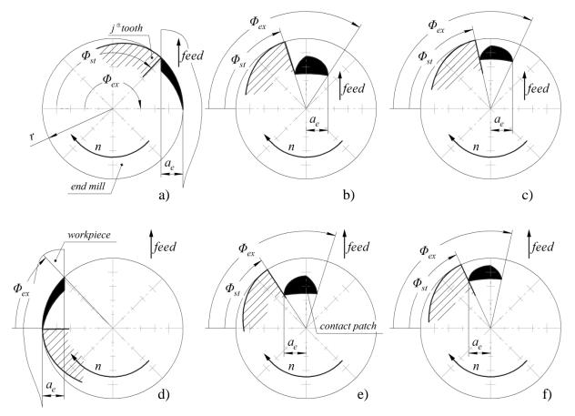
**Fig. 1** Start and exit angles in end mill machining, a) down-milling with flat end mill, b) down-milling with ball end mill (lead angle 30°), c) down-milling with ball end mill (lead angle 45°), d) up-milling with flat end mill, e) up-milling with ball end mill (lead angle 30°), f) up-milling with ball end mill (lead angle 45°)
