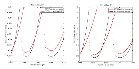
Fig. 6 Comparison of classical approach and proposed method for stability lobes in slot-milling with  $30^{\circ}$  and  $45^{\circ}$
