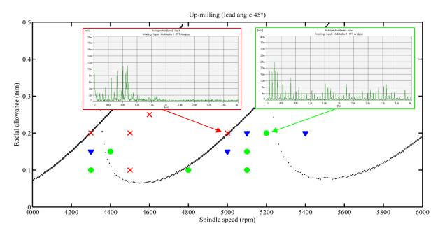
Fig. 14 Experimental stability for up-milling (lead angle  $45^{\circ}$ ), stable tests results are marked with green  $\circ$ ; limited stable tests results are marked with blue  $\nabla$ ; unstable tests results are marked with red  $\times$
