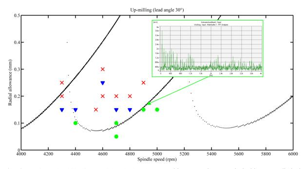
Fig. 13 Experimental stability for up-milling (lead angle 30°), stable tests results are marked with green  $\circ$ ; limited stable tests results are marked with blue  $\nabla$ ; unstable tests results are marked with red  $\times$
