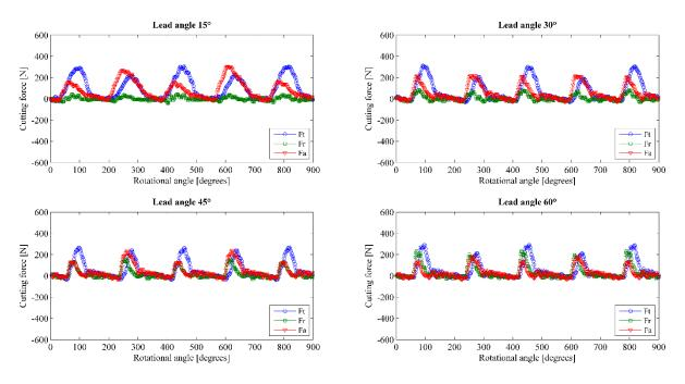
Fig. 9 Cutting force components for various lead angles (15° 30° 45° 60°) in slot-milling
