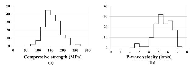
Fig.5. Histograms of compressive strength  $f_{c}\left(a\right)$  and ultrasonic P-wave velocity  $V_{p}\left(b\right)$
