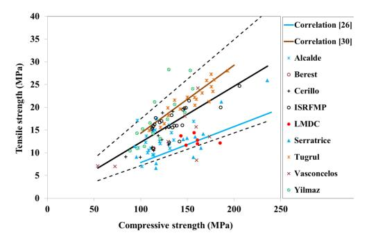
Fig.13. Tensile strength, fct, versus compressive strength, fc.
