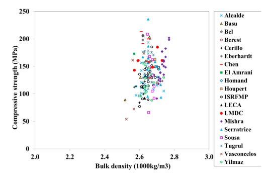
Fig.6. Compressive strength, fc, versus bulk density, p
