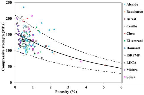
Fig.7. Compressive strength, f<sub>c</sub>, versus porosity, P<sub>o</sub>
