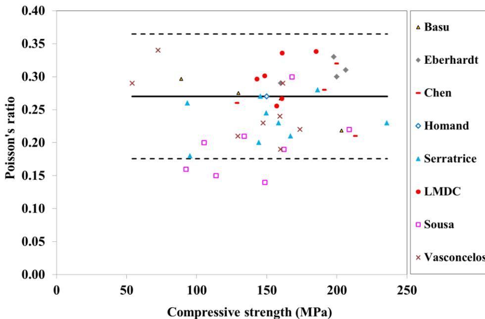
Fig.10. Poisson's ratio,  $\nu$ , versus compressive strength,  $f_c$
