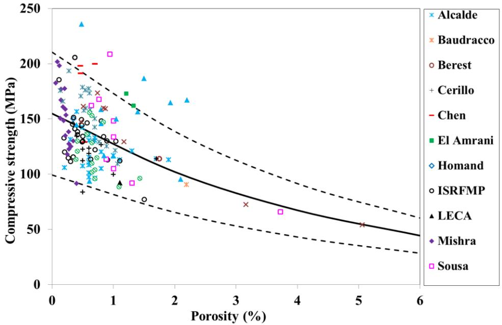
Fig.7. Compressive strength,  $f_c$ , versus porosity,  $P_o$
