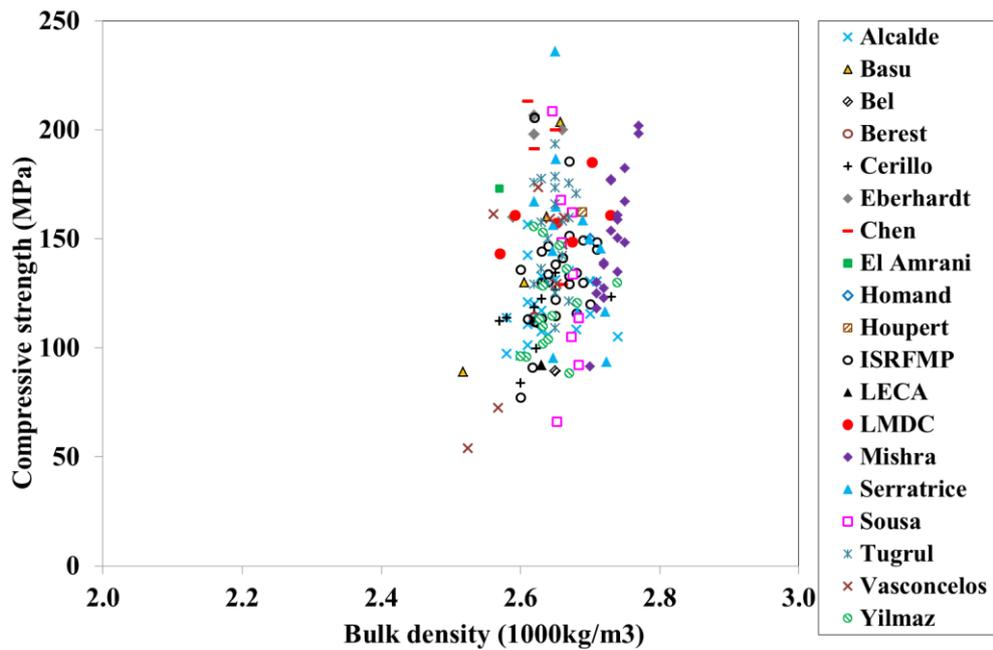
Fig.6. Compressive strength,  $f_c$ , versus bulk density,  $\rho$
