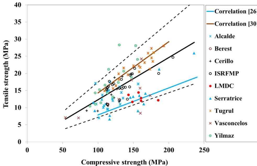
Fig.13. Tensile strength,  $f_{ct}$ , versus compressive strength,  $f_c$ .
