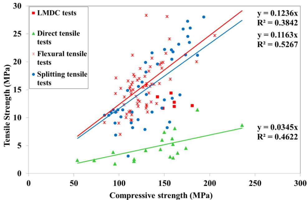
Fig.12. Tensile strength versus compressive strength,  $f_c$ , according to type of test
