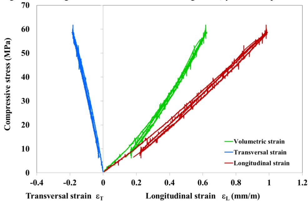
Fig.4 – Stress-strain curves with 3 loading-unloading cycles (specimen E)
