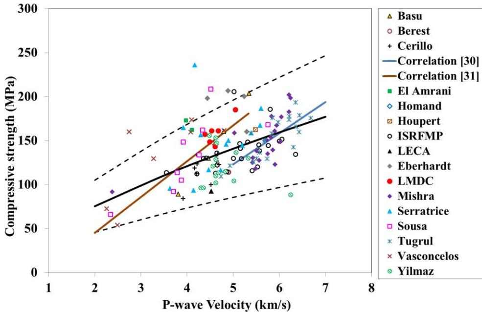
Fig.8. Compressive strength,  $f_c$ , versus P-wave velocity,  $V_p$
