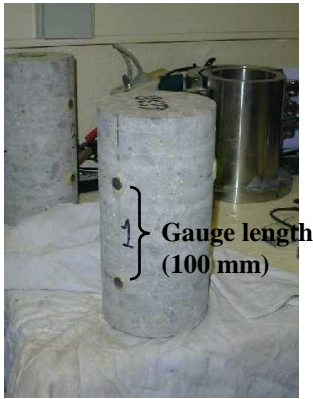
Fig. 2: Cylindrical specimens equipped with balls for extensometer measurement
