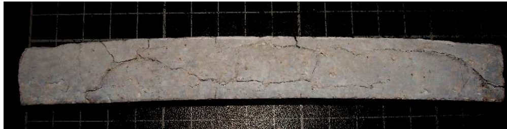
15 Figure 11: Cracking patterns of specimens cast with opal (20x20x160 mm)
