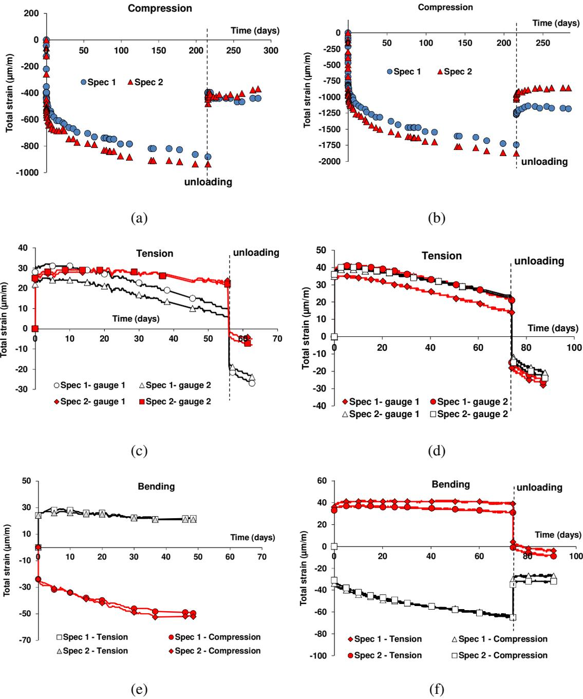
642 Figure 5: Total strains (elastic strains included) in compression at 30% and 50% of  $f_c$  (a and
