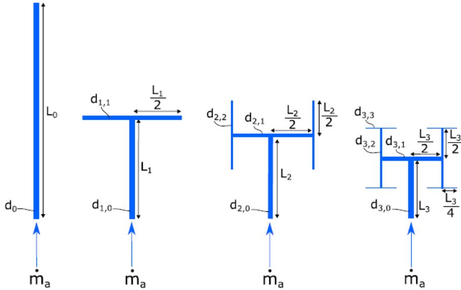
FIGURE 4. Network shape for bifurcation level  $N$  ranging from 0 (left, corresponds to the straight pipe) to 3 (right). The overall fluid volume is fixed. The networks are drawn to scale in accordance with the results of Section 3.2.
