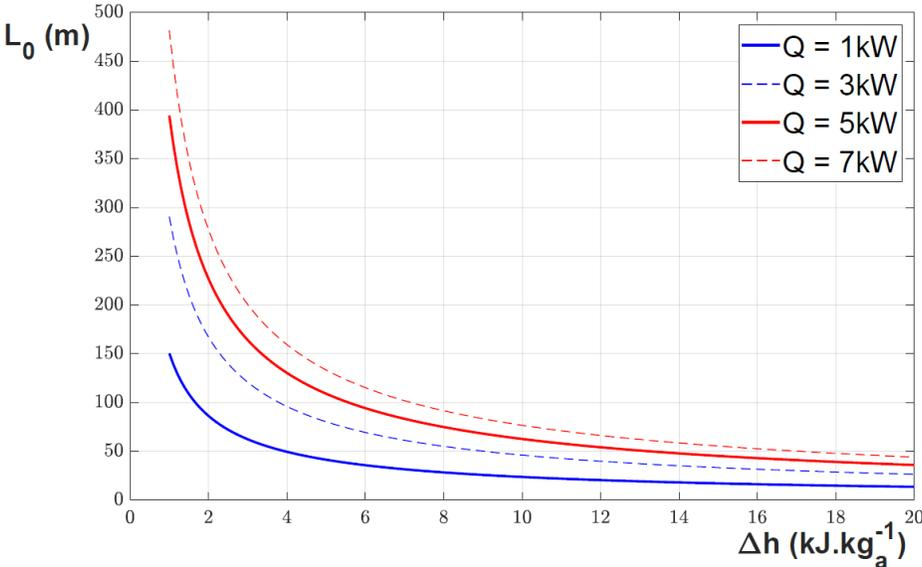
FIGURE 3. Pipe length as a function of the enthalpy difference ( $\Delta\mathbf{h} = \mathbf{h}_{\text{in}} - \mathbf{h}_{\text{w}}$ ) for different values of the targeted cooling power
